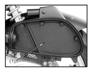
Wash the air cleaner element in detergent oil, squeeze out and allow to dry.
