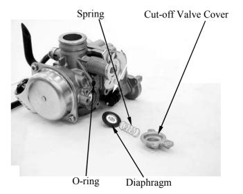
Install and tighten the two screws attaching the air cut-off valve cover.
