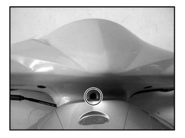
Remove the two screws from the handlebar rear cover.
