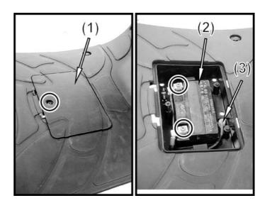
Remove the four bolts and then remove floor board.
