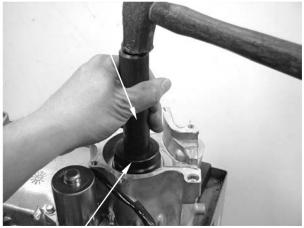
Bearing Outer Driver, 42x47mm Pilot, 20mm
