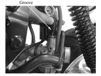
Tighten the carburetor top. After installation, perform the following adjustments and inspections.
