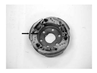
Measure the driven face spring free length. **Service Limit**: 82.6mm replace if below
