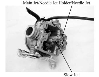
Clean the removed the main jet, needle jet holder, needle jet and slow jet with detergent oil.
