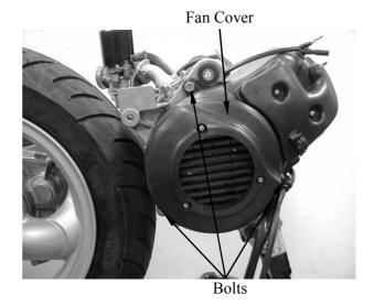
Remove the cooling fan by removing the four bolts.
