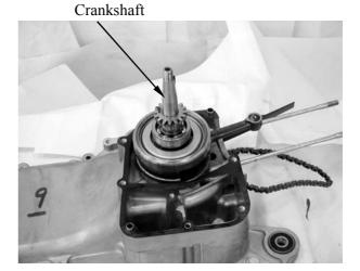
Remove the cam chain. Remove the gasket and dowel pins.
