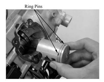
Lubricate the cylinder inside and piston rings with engine oil and install the piston into the cylinder while compressing the piston rings.
