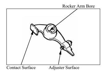
Measure each rocker arm shaft O.D. Measure the I.D. of each valve rocker arm. Measure arm to shaft clearance. Replace as a set if out of specification.
