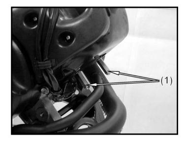
Remove the bolt from the rear lower fender and two Exhaust muffler lock bolts from the exhaust muffler.
