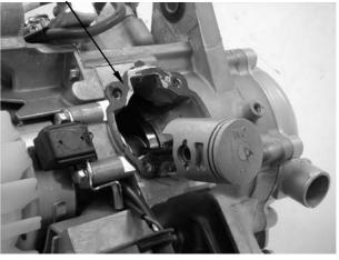
Make sure that the ring end gaps are aligned with the piston ring pins in the ring grooves.
