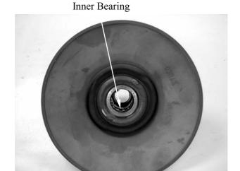
Remove the snap ring and drive the outer bearing out of the driven face.
