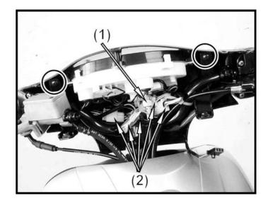
Remove the three screws from the instrument and then remove handlebar rear cover.
