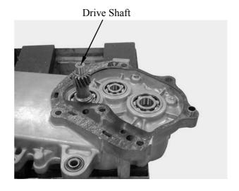
Install the final gear and final shaft into the left crankcase.
