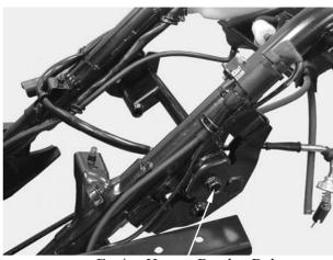
Engine Hanger Bracket Bolt
