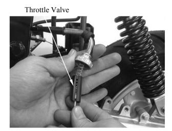
Remove the throttle valve spring, carburetor top and rubber seal.
