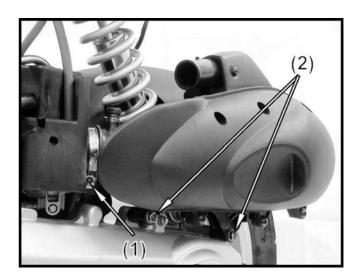
Slide the rubber sleeve up to expose the carburetor.
