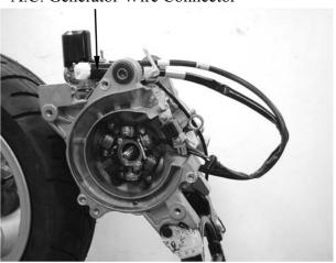
Remove the two pulser coil bolts and pulser coil from the right crankcase.
