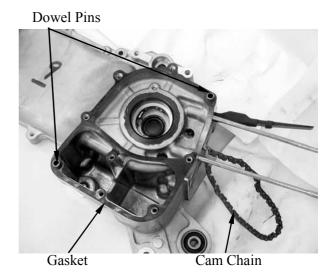
Clean off all gasket material from the crankcase mating surfaces.
