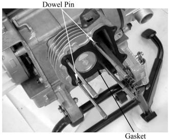
Remove cam chain guide and then remove cylinder.
