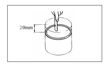
Measure the piston pin hole I.D.
