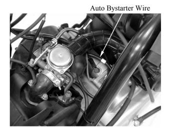
Disconnect the fuel tube from carburetor.
