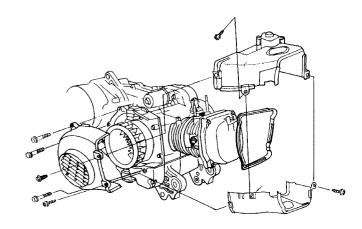
Remove seal shroud, then remove two bolts and cylinder head.
