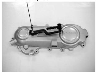
Slightly rotate the kick starter spindle to remove the kick starter driven gear together with the friction spring.
