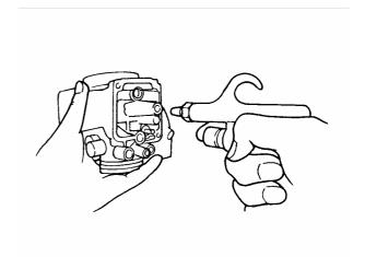
Install the O-ring onto the air-cut-off valve body securely.
