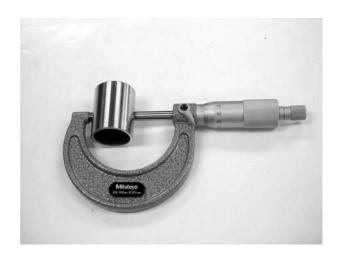
Check the caliper cylinder for scratch or wear and measure the cylinder bore.
