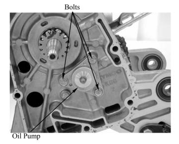
Install the oil pump gear and tighten the nut.
