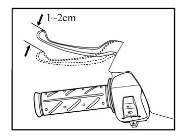
Place the scooter on its center stand. Turn the adjusting nut in direction (A) to decrease play, and in direction (B) to increase play.
