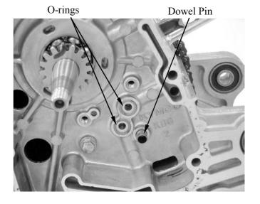
Install the oil pump and tighten the bolts. Make sure that the pump shaft rotates freely without binding.
