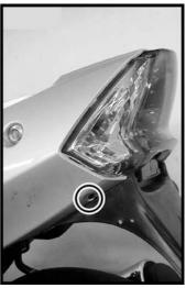
Remove the two screws form the rear body cover
