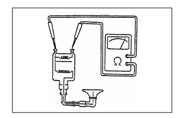
Measure the secondary coil resistance between the spark plug cap and the primary coil terminal as Figure A shown.
