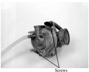
Remove the screw and O-ring. Remove the float pin, float and float valve.
