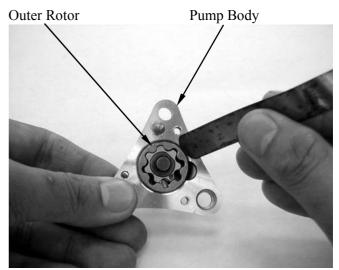
Measure the inner rotor-to-outer rotor clearance.
