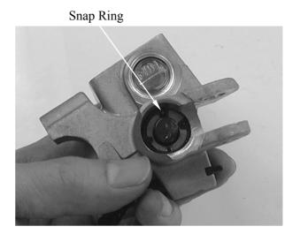
Remove the washer, main piston and spring from the brake master cylinder. Clean the inside of the master cylinder and brake reservoir with brake fluid.
