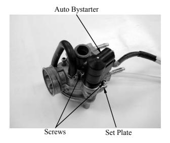
Check the auto bystarter valve and needle for wear or damage.
