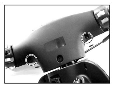
Disconnect the winker relay from the handlebar front cover and then remove handlebar front cover.
