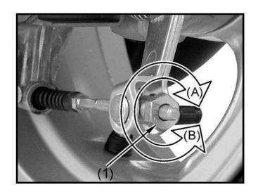
Make sure the cut-out on the adjusting nut (2) is seated on the brake arm pin (1) after making final free play adjustment.
