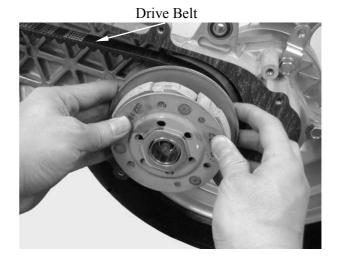
Set the drive belt on the drive pulley. Install the drive pulley face, starting ratchet and 12mm drive face nut, then tighten the drive face nut.
