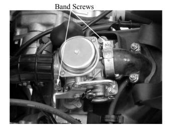
Connect the throttle cable to the carburetor.
