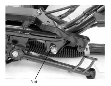
Remove the engine hanger bracket bolts and engine hanger bracket.
