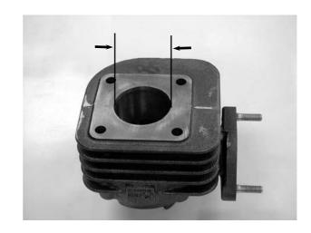
Inspect the top of the cylinder for warpage. **Service Limit**: 0.10mm replace if over
