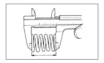
Measure compressed force (valve spring) and installed length.
