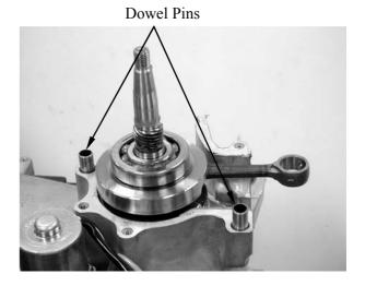
Assemble the crankcase halves.
