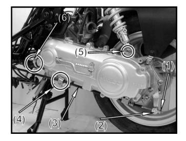
Remove the secondary air hose band (1) from the exhaust muffler and disconnect the secondary air hose.
