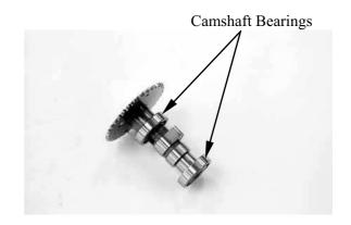
Inspect camshaft lobes for pitting/scratches/blue discoloration.
