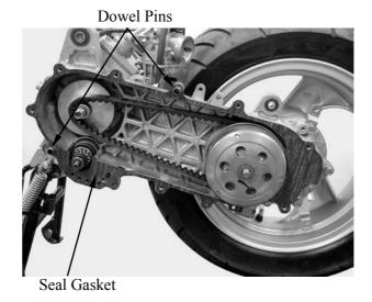
Install the left crankcase cover and tighten the ten bolts diagonally.
