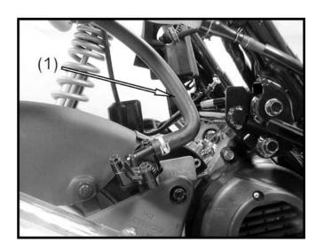
Remove the right and left engine mounting nuts (1).
