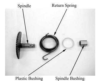
Check the kick starter driven gear for wear or damage.
