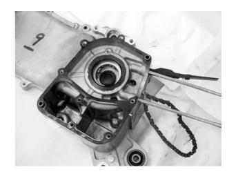
Install the crankshaft into the left crankcase.
