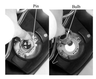
Install a new bulb in the reverse order of removal.
