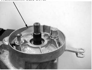
Install and tighten the transmission case cover bolts.
