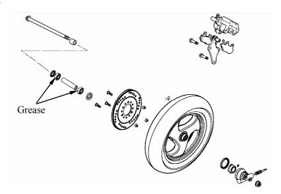
Pack all bearing cavities with grease. Drive in the left bearing. Install the distance collar. Drive in the right bearing.
