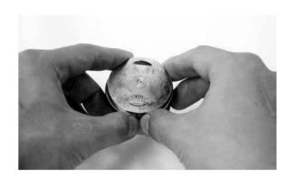
Inspect the piston wall for wear/scratches/damage.
