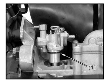
Install the oil pump into the crankcase. Install the oil pump control cable plate (1) and tighten the two bolts.
