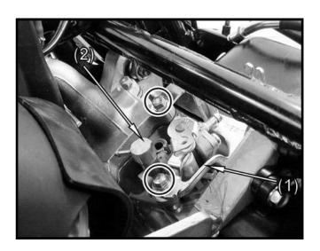
Connect the oil inlet line (1) and oil outlet line (2) properly.
